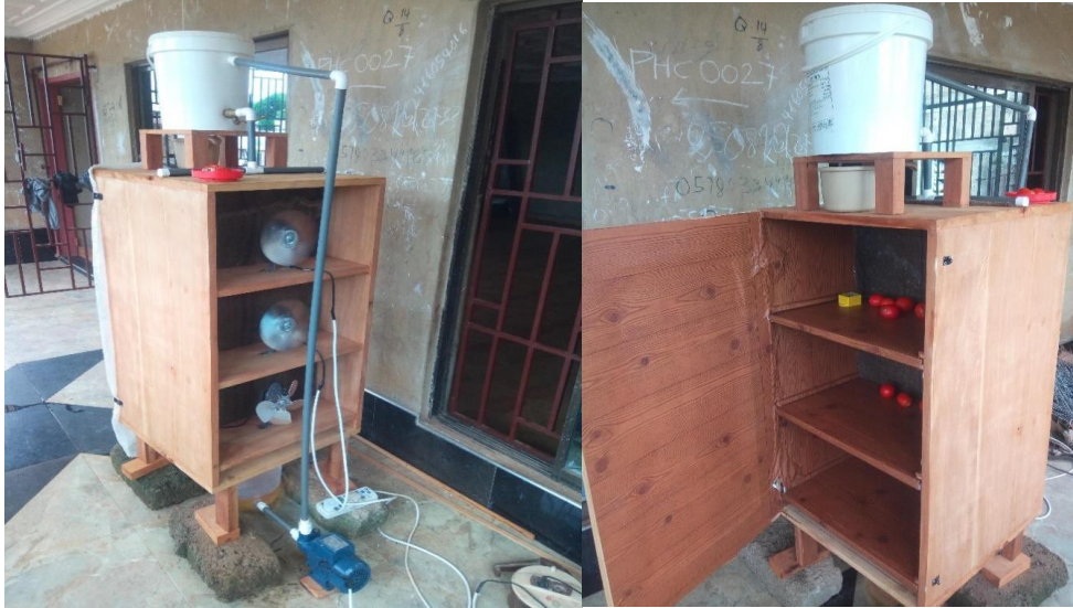
Figure 3. General overview of the evaporative cooler
