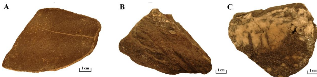
Fig.6. A - Sericized carbonaceous-siltstone rock; B - Carbonaceous siltstone rock with polymetals; C – Sulfide-rich carbonaceous siltstone with quartz–antimonite veins. (The samples of “A” and “B” from Bakyrchik deposit, and the “C” sample from Bolshevik deposit). (modified after a camera 5MP and Photo Shop CS3)
