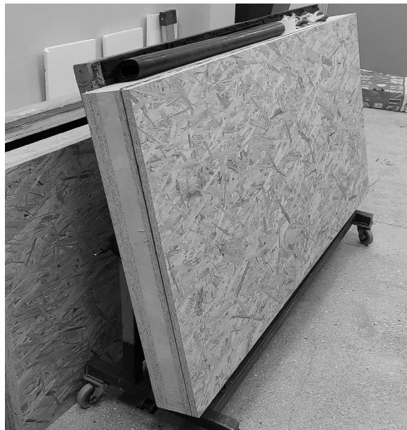
Figure 2. Second partition (B) without measuring hole.
