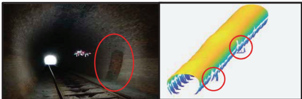
Fig. 3. Tunnel inspection: (a) a UAV during inspection [30], (b) a 3D point cloud of a tunnel with cavities [38]
