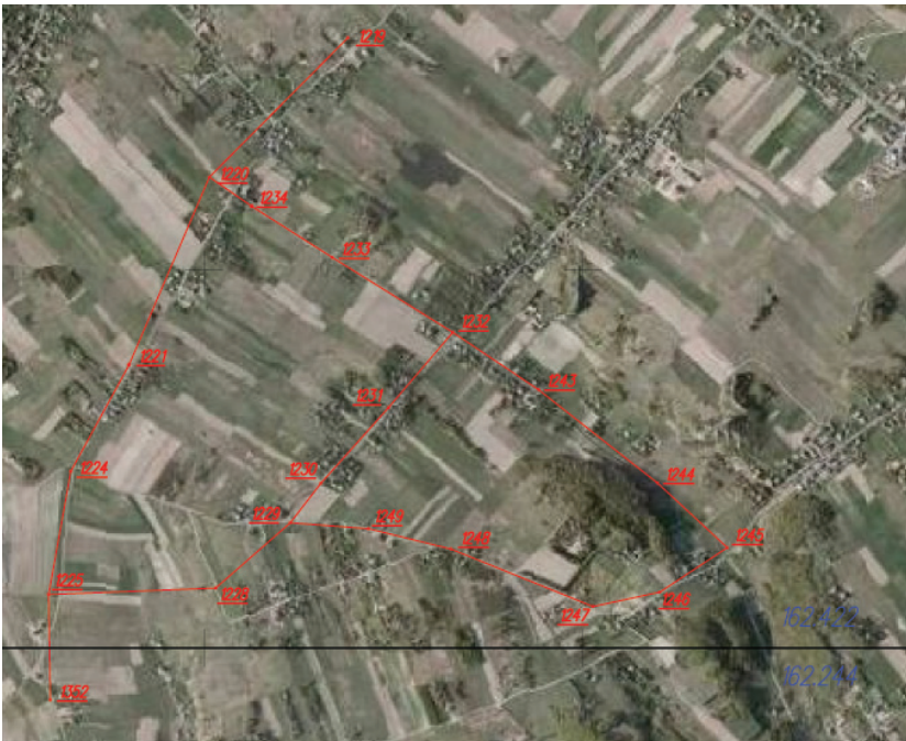
Fig. 5. Sketch of a fragment of the 3rd class detailed control network (test network) in “Jerzmanowice-Przeginia” area
