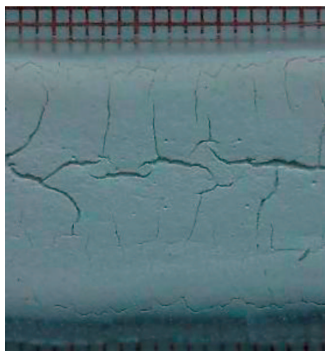
Fig. 4. An image of thin layer made of 54vol.% alumina suspensions with addition of 25wt.% polyester resin, obtained by tape casting method and cured by UV irradiation
