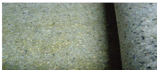
Fig. 10. Agronomic fabric for cultivation with fertilizer made from fabaceae
