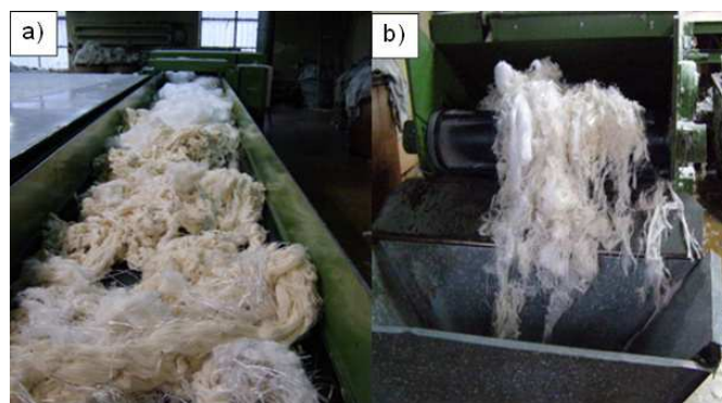
Fig. 3. Rotary cutter: a) input, b) output
