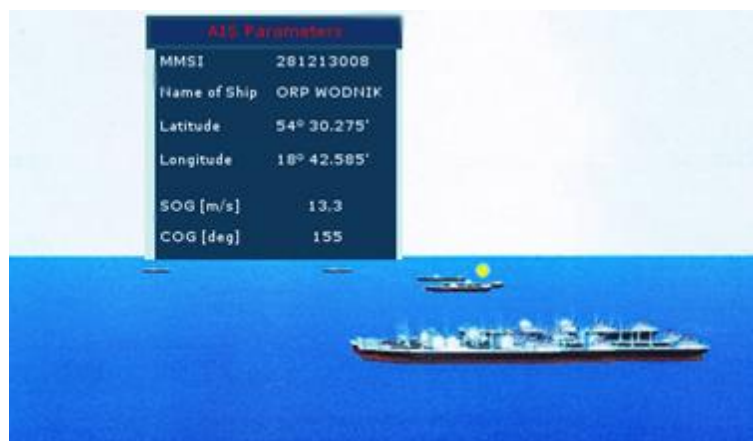
Fig. 15. Window with the parameters of the indicated vessel in the AR display system
