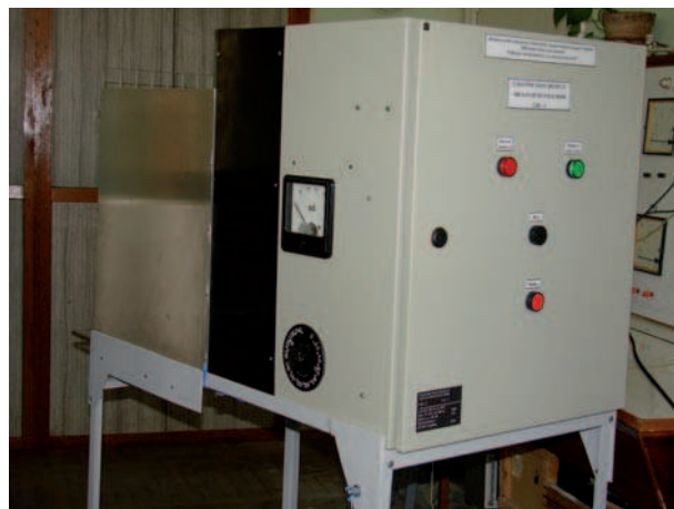
Fig. 1. Appearance settings for the processing of cereals in the electric field of high intensity
