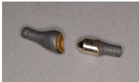
Fig. 1a. Sample of primary cast crown and secondary electroformed coping prepared for testing
