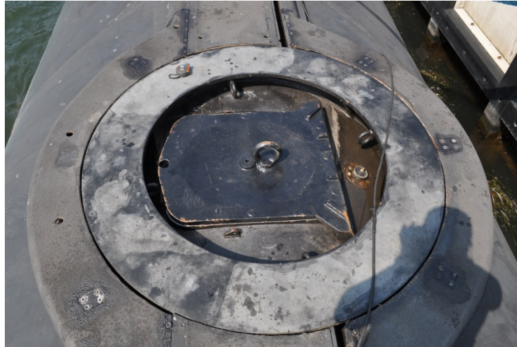
Pic. 1. Rescue seat area of submarine Kobben class (ORP Sokół) [2]
