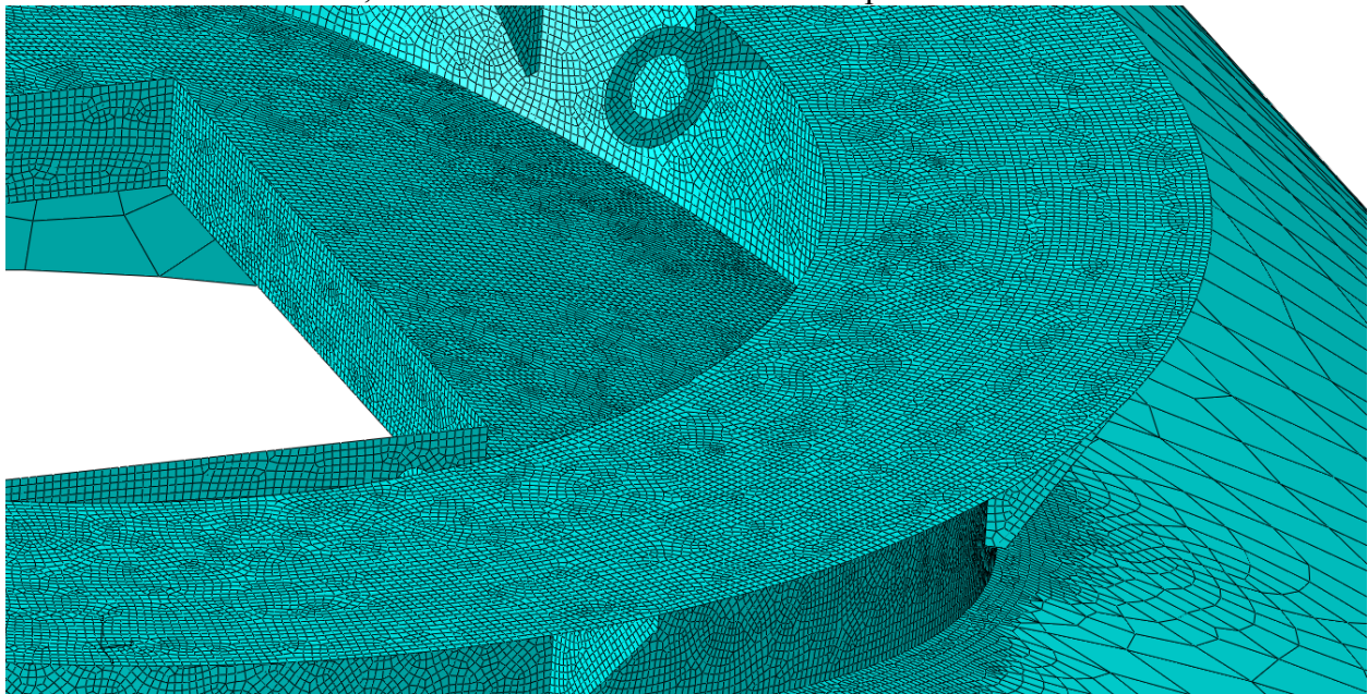
Pic. 5. Solid geometry discretization of rescue seat area
