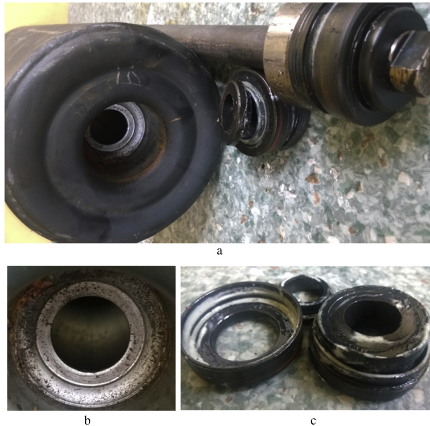
Fig. 12. The \phi 133 \times 465 idler with a labyrinth seal and a deflector: a – the idler after the water-tightness test, b – inside of the hub, visible rust spots and mildew stains, c – the seal with the remains of washed out grease.
