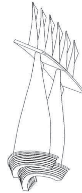
Figure 3. Fork-shaped blade of two-tier stage.
