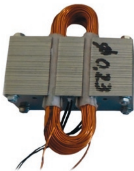
Fig. 10. Sample of the electromagnetic circuit
