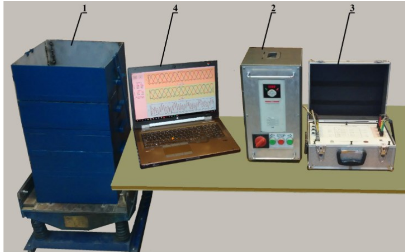
Fig. 2. The research system: 1 – model vibratory unit, 2 – inverter, 3 – instantaneous voltages and currents values recorder, 4 – computer with recorder’s software
