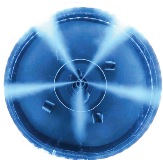
Fig. 20. Fuel spray pattern of a damaged injector
