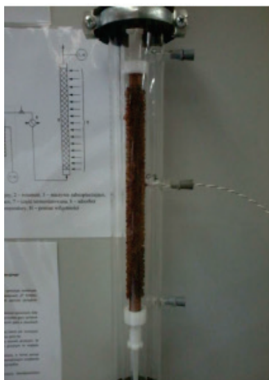
Figure 2. A glass adsorber with a silica gel-coated copper pipe
