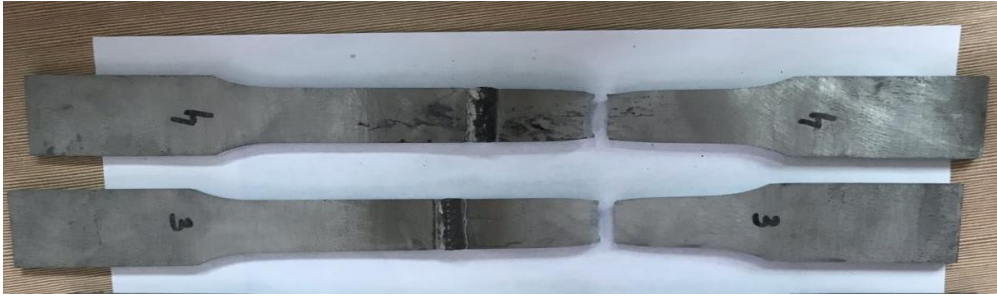
Fig. 4. Examples of samples for which the crack occurred in base material
