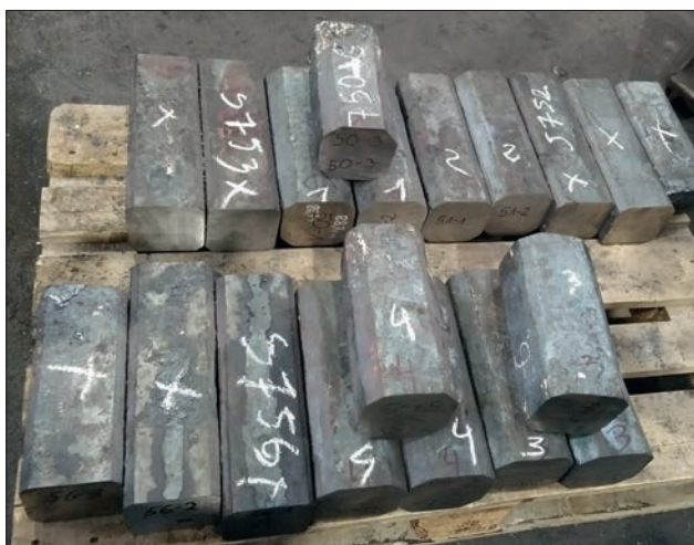
Fig. 8. Sections of bars intended for forging for semi-finished products for bodies
