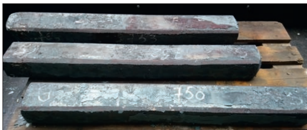
Fig. 7. 110 square bars after free forging
