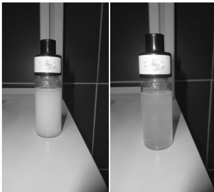
Fig. 3. On left- sample after 10 minutes of demulsifier addition. On right- sample after 180 minutes of demulsifier addition.
