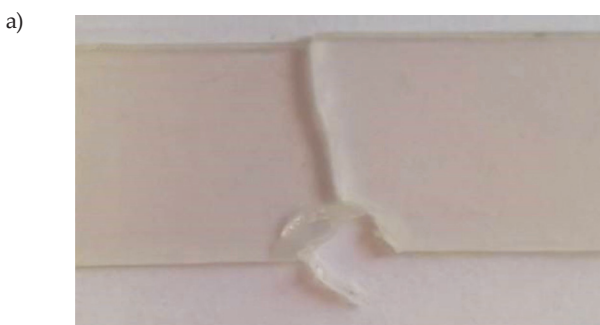
Fig. 10. Images of a sample after impact resistance determination: a) PET-G, b) specimen E (composite PET-G with 20 wt % of PET)
