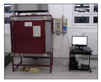
Fig. 4. The bench for heating the samples Source: [Own study].
