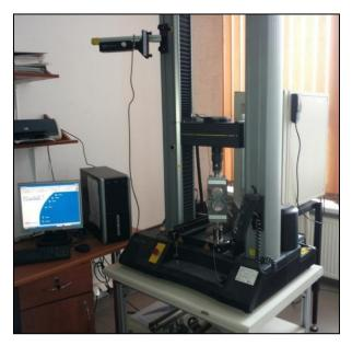
Fig. 7. The bench for testing the tensile strength Source: [Own study].
