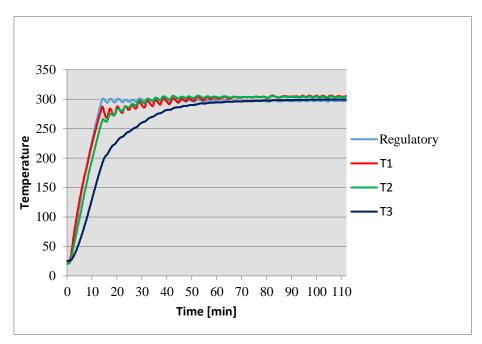
Fig. 6. The heat-soaking process – the temperature of 300°C Source: [Own study].
