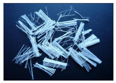
Fig. 2. The polypropylene fibers Fortatech® Fibre High Grade Source: [Own study].
