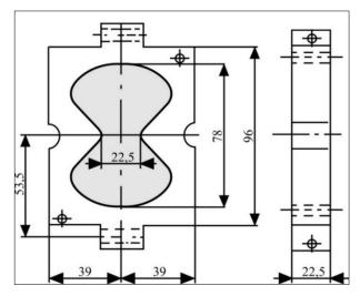
Fig. 3. The steel mold for the preparation of octal specimens for testing Source: [Own study based on: PN-B-04500:1985]
