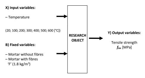
Fig. 1. The research program for determining the tensile strength  $f_{tp}$ Source: [Own study].
