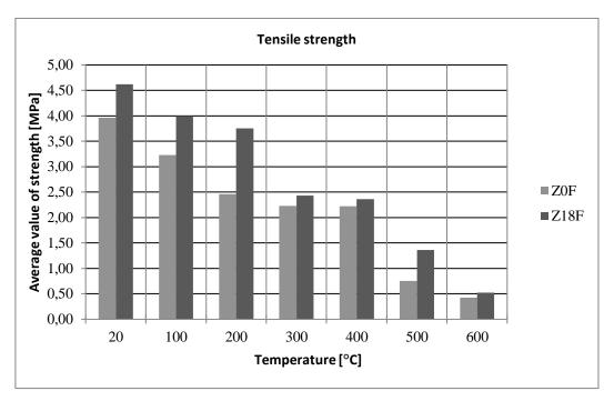
Fig. 8. The summary of average tensile strengths of concrete samples without and with the addition of polypropylene fibers at different temperatures *Source: [Own study].*
