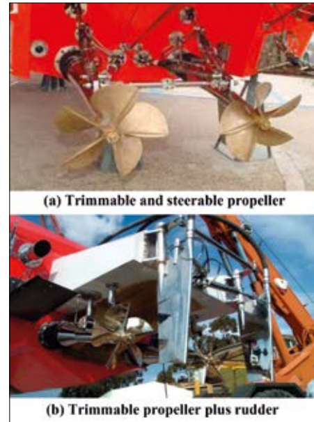
Fig. 4. Steering system of the planing craft [26]
