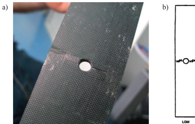
Fig. 2. Failure Mode that occurred at the specimen 001 (AUD) during the OHC test (a) and equivalent ASTM failure mode LGM (b)
