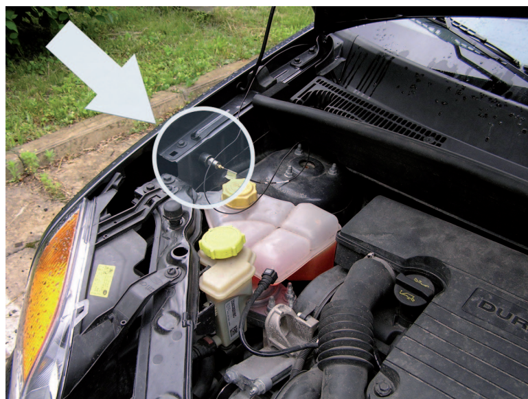
Figure 4. Positioning a vibration sensor, acting as the reference source in the engine compartment of a Ford Fusion.
