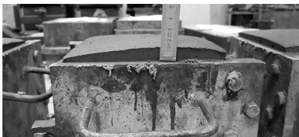
Fig. 1. The expansion of the samples after 60 minutes from contact of cement with water
