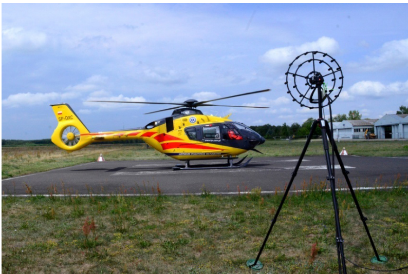
Fig. 2. Measurement with the acoustic camera to determine the sources and noise spectrum of the helicopter [W. Krzymień, 2018].
