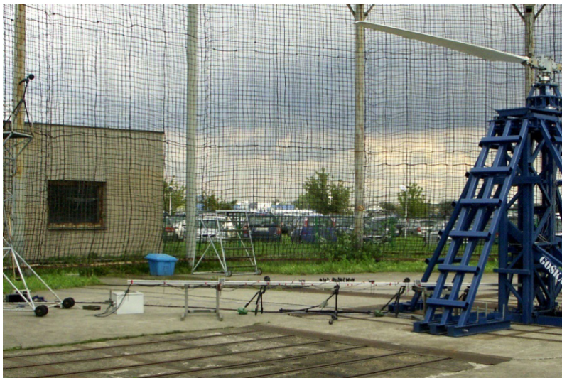
Fig. 7. The stand for investigation of helicopter main rotors [W. Krzymień, 2018].
