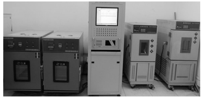
a) Physical map of relay testing system
