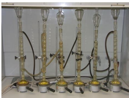
Fig. 2. Extraction device with a reflux condenser
