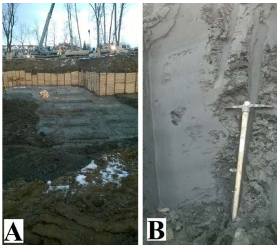
Text-fig. 2. Location of sampling glacial till samples: A – general view of the excavation, B – view of the excavation wall with visible glacial till
