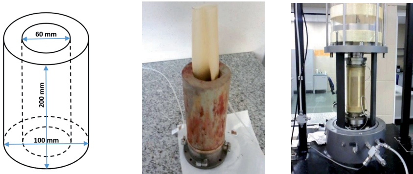
Fig. 7. Soil sample in the shape of hollow cylinder prepared for testing in a torsional shear hollow cylinder apparatus [34]
