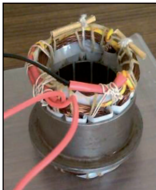
Fig. 2. Dissembled view of the MR damper
