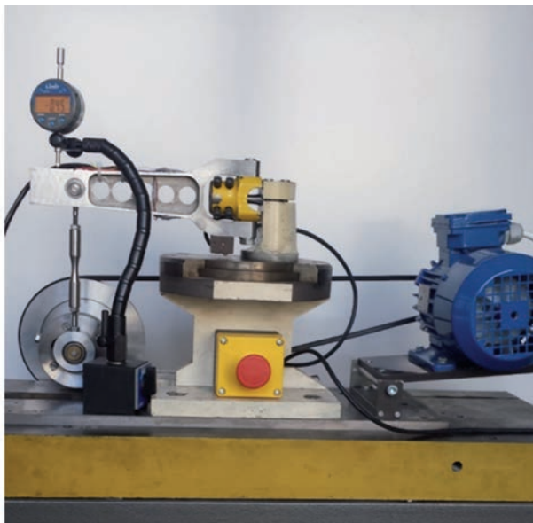
Fig. 7. The setup for fatigue tests under controlled strain
