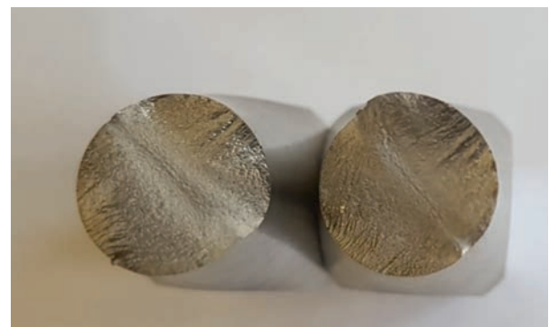
Fig. 8. An example test piece photo taken after oscillatory bending test
