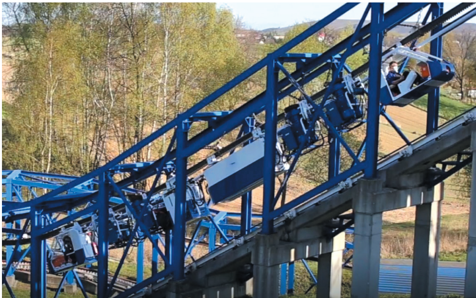
Fig. 6. Basic configuration of the CA-190/4/2/2 locomotive on a test track – the track inclination is 30 degrees
