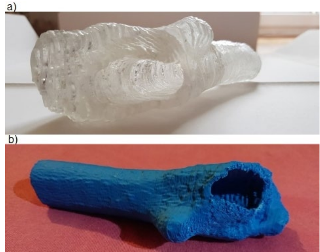
Figure 6. A physical model of the fragment of the femur made using (A) stacked layers method and (B) 3D printing.
