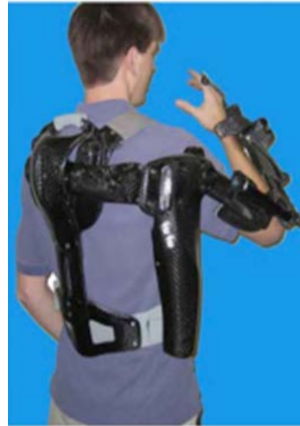
Figure 8. Upper limb rehabilitation manipulator exoskeleton - Rupert II (left) and Rupert III (right) [7].
