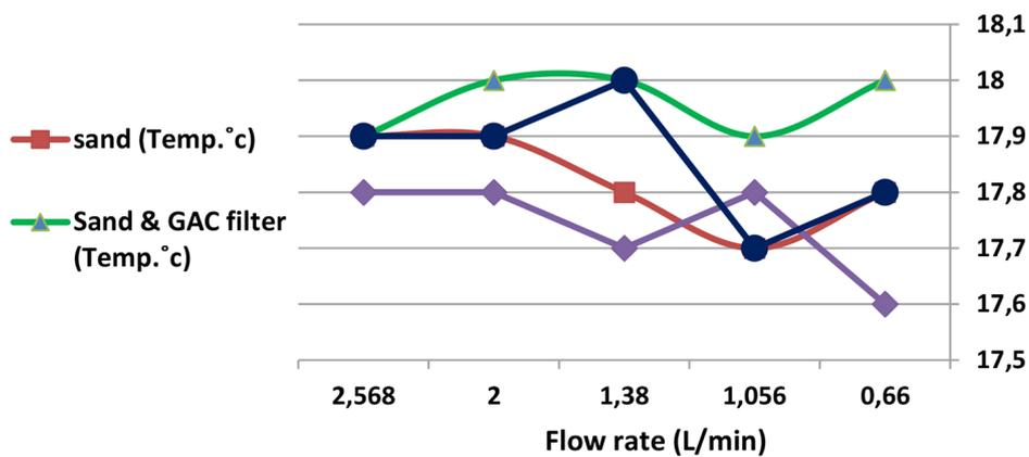
**Figure 4.** Variation in temperature parameter with flow rate of treated and raw storm water
