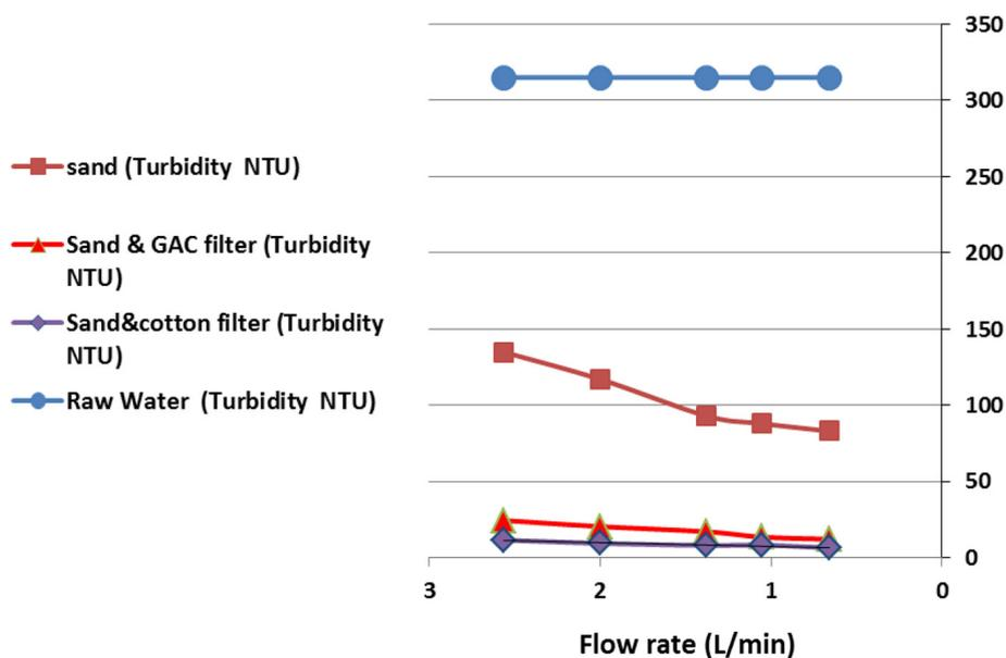
Figure 8. Variation of turbidity with flow rate of treated and raw storm water
