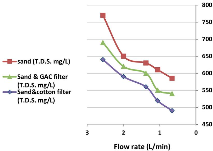
Figure 7. Variation of TDS with flow rate for treated and raw storm water
