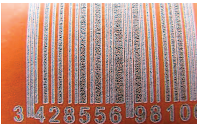
FIG.5. EXAMPLE OF BAR CODE ON CARDBOARD GC-2 (MODES OF LASER MARKING: POWER P=14\text{ W} , RATE V=240\text{ MM/S} )
