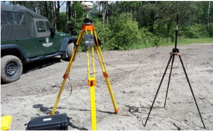
Fig. 9. Mobile reference station (Trimble R4 and Satel-TA18 radio)
