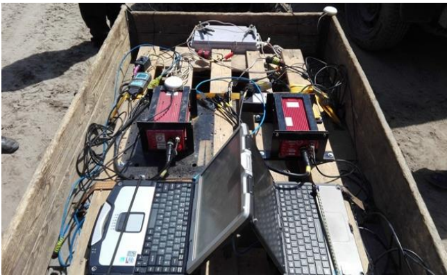
Fig. 10. The RT4000 device mounted on a single-axis trailer
