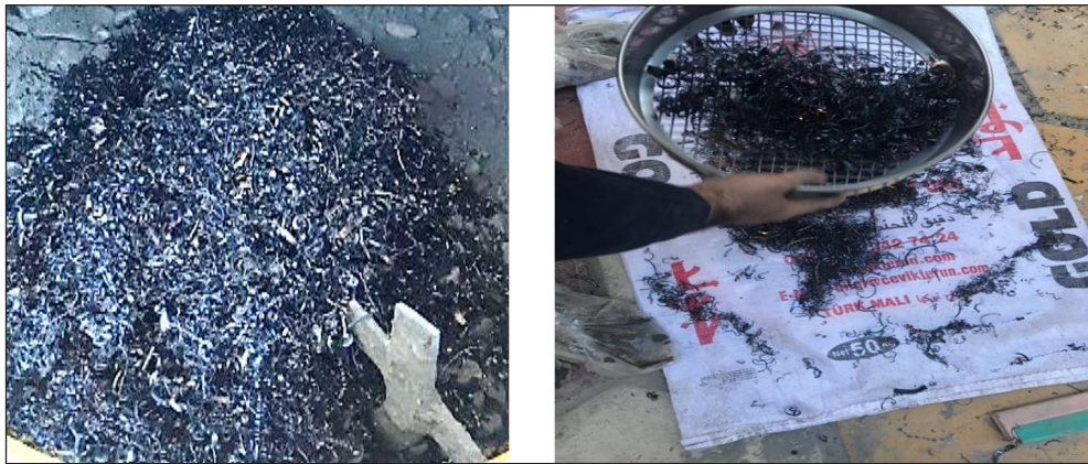
Figure 1. Technique for processing recycled steel fiber
