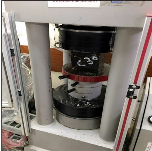
Figure 3. Compressive strength test
