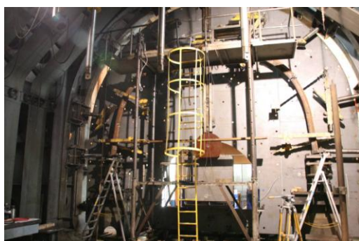
Photo 2. ŁPw support arch in test stand during tests
