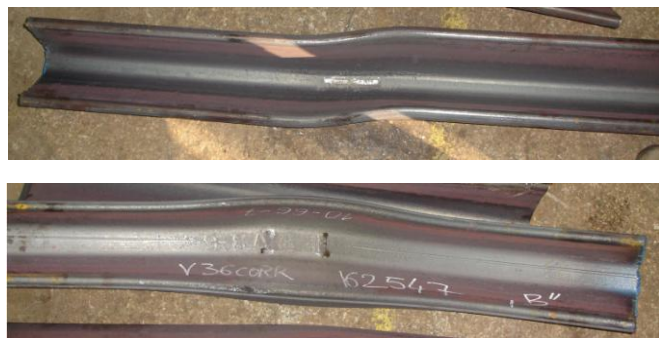
Photo 1. Profiles after bend test 'bottom down' (top) and 'bottom up' (bottom)
