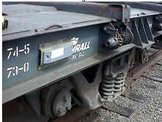
Fig. 2. Platform-mounted RFID tag
