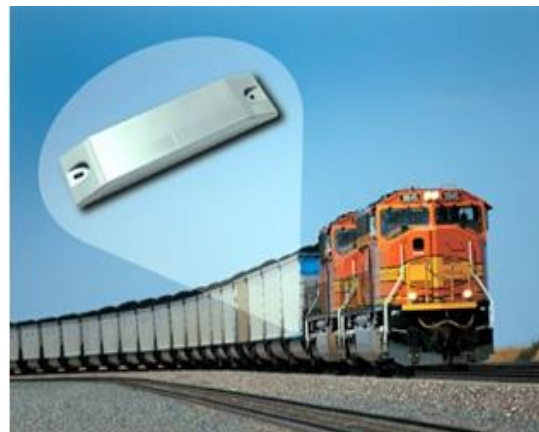
Fig. 1. Train car mounted RFID tag
