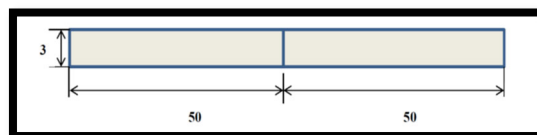
Fig. 1. Dimensions of samples to be joined (in millimetres)
