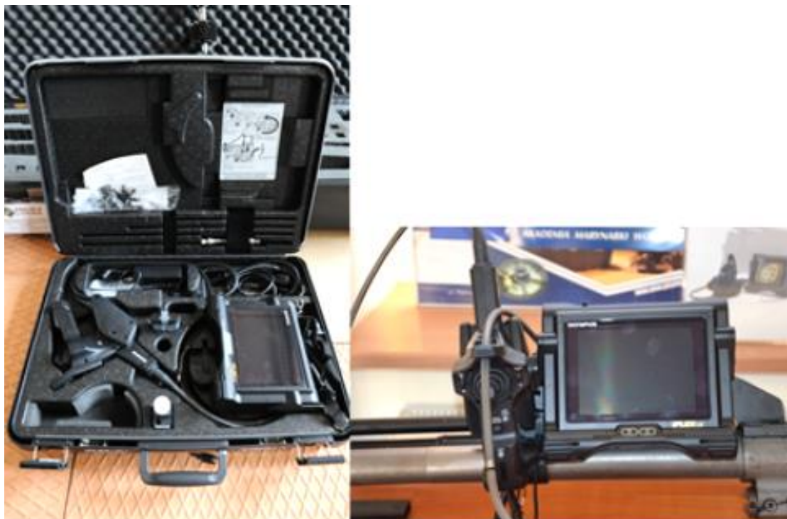
Fot. 12. Wideoskop IPLEX LX do diagnostyki lufy 35 mm AM Photo 12. Videoscope IPLEX LX for diagnosis of 35 mm naval gun barrel
