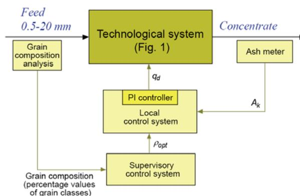
Fig. 2. Block diagram of a control system for one of two jigs (as in Fig. 1)
