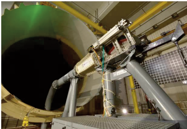
Picture 3. Wind tunnel with secondary flow capability during test setup for a thrust reverser test.
