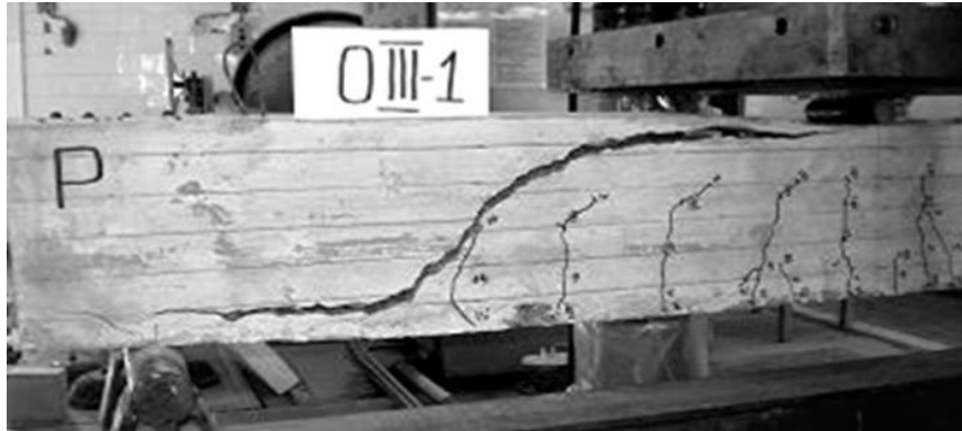
Fig. 3. Diagonal failure in a beam without transverse reinforcement
