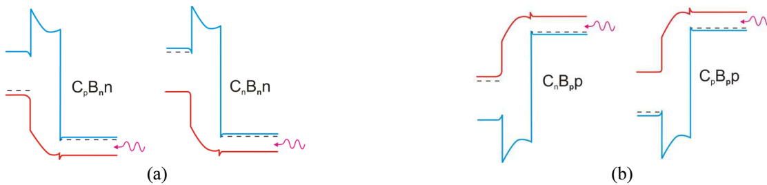
Fig. 3. Schematic band profile configurations for n-type base (a) and p-type base (b) barrier detectors.
