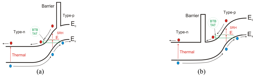
Fig. 5. Theoretical band diagrams of p-n photodiodes with barriers in the p-type (a) and the n-type (b) region.
