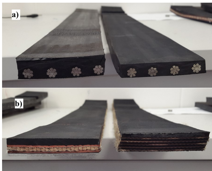
Fig. 3 Conveyor belt samples: a – steel-cord belts, b – textile belts - aramid single-ply belt and multiply belt
