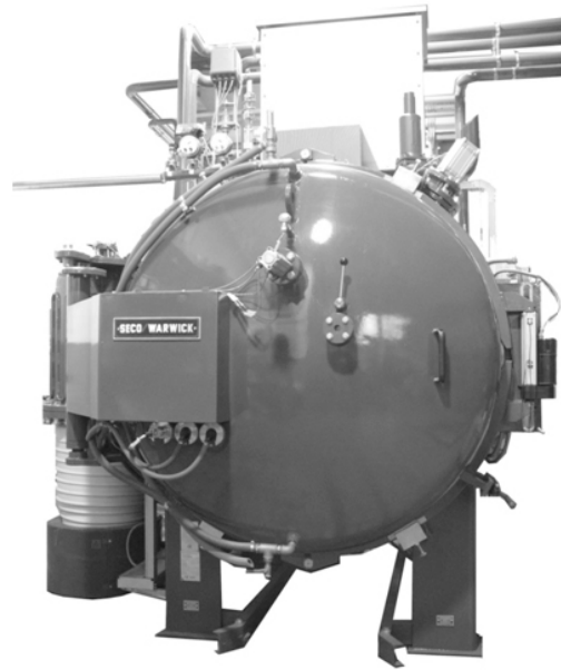
Fig. 6. A universal vacuum furnace with gas cooling operating at the Institute of Precision Mechanics in Warsaw
